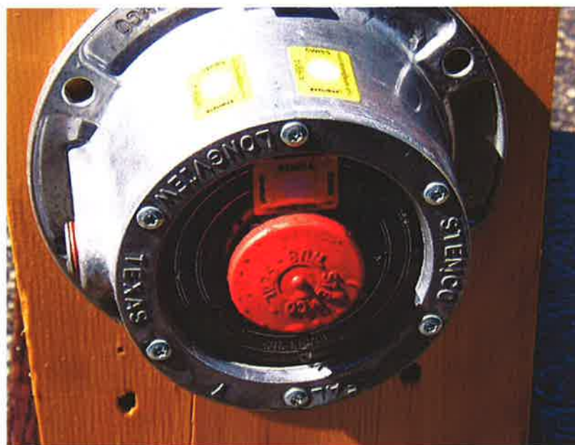
Figure 13A : Aluminum hub cap with labels – Hot temperature, after pressure spraying
