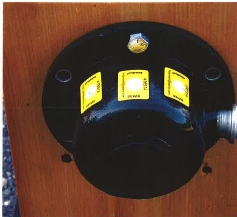
Figure 20A : Plastic hub cap with labels – Cold temperature, after pressure spraying
