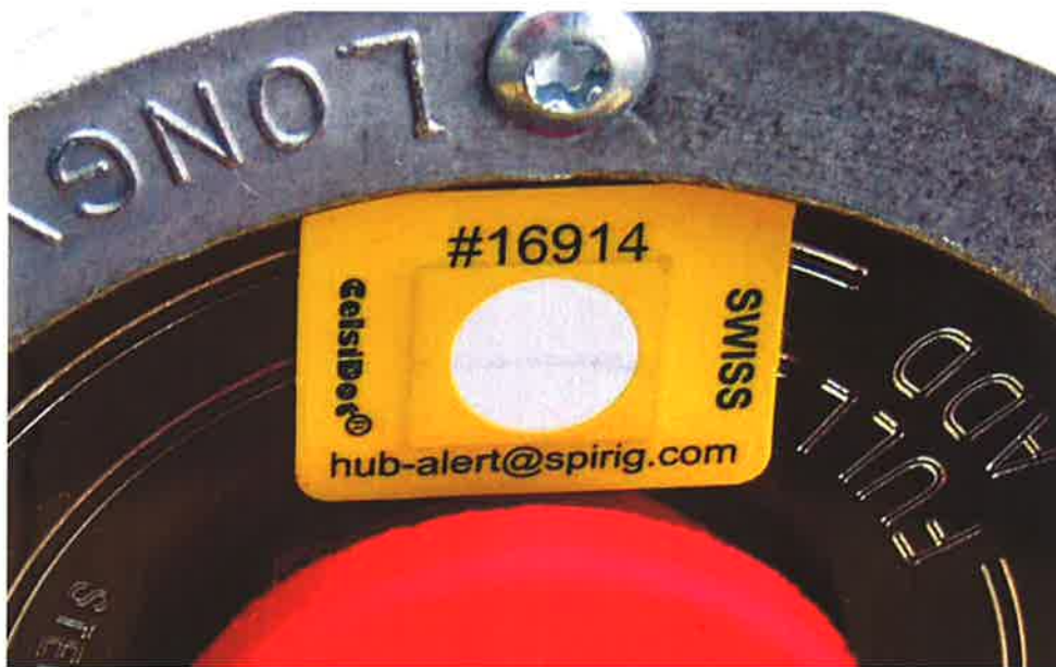
Figure 7A : Aluminum hub cap with labels – Ambient temperature, after pressure spraying
