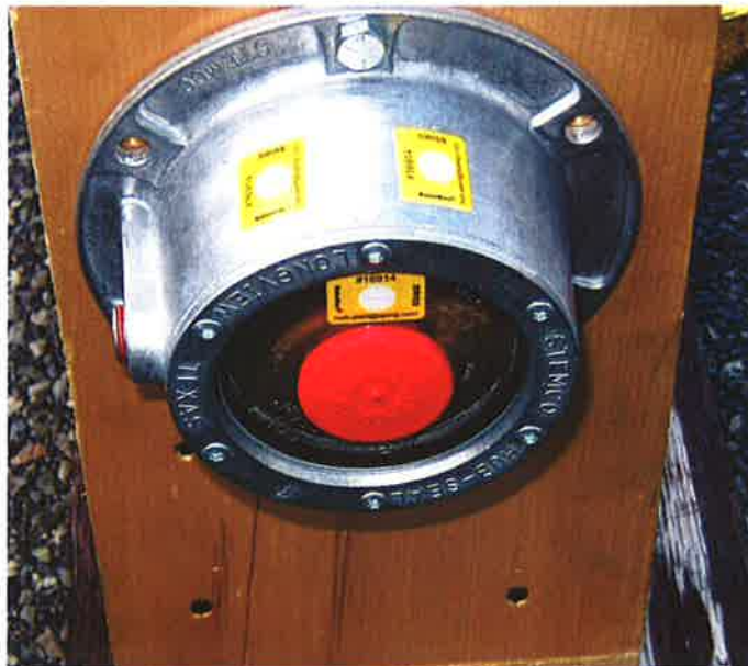
Figure 4A : Aluminum hub cap with labels – Ambient temperature, before pressure spraying
