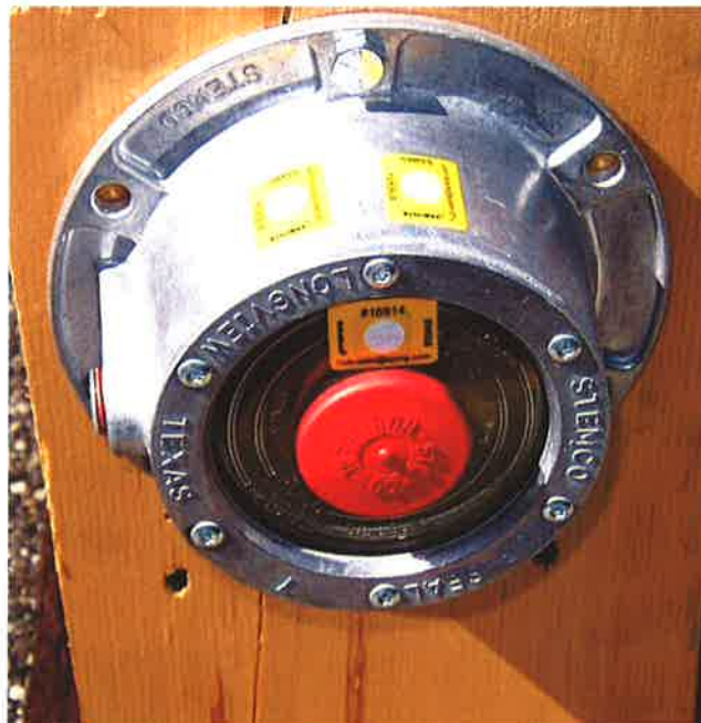
Figure 10A : Aluminum hub cap with labels – Hot temperature, before pressure spraying
