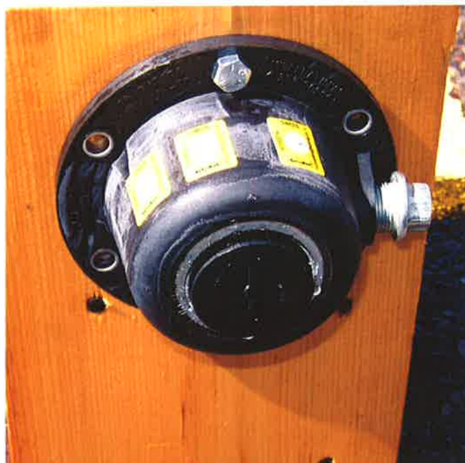
Figure 14A : Plastic hub cap with labels – Hot temperature, after pressure spraying
