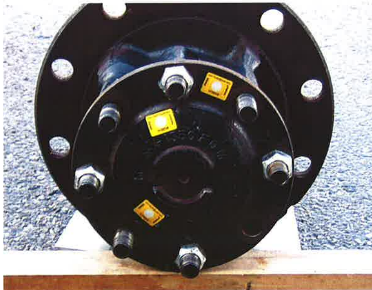
Figure 6A : Steel hub cap with labels – Ambient temperature, before pressure spraying
