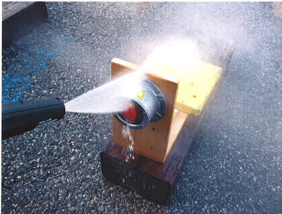
Figure 2A : Pressure-washer resistance test set-up
