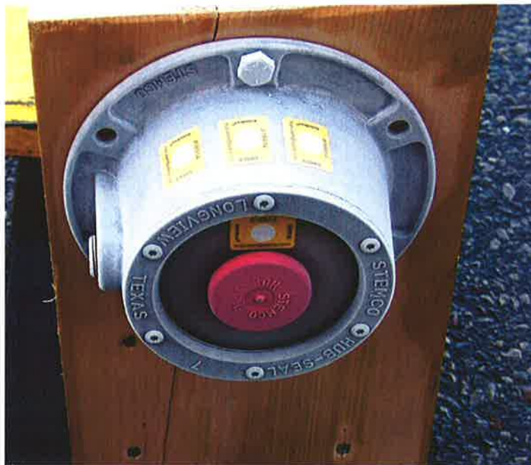
Figure 16A : Aluminum hub cap with labels – Cold temperature, before pressure spraying
