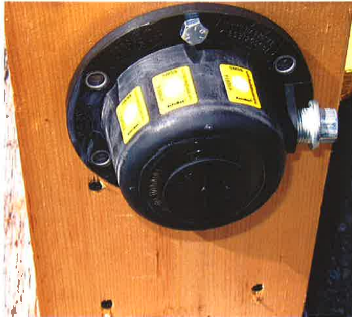
Figure 11A : Plastic hub cap with labels – Hot temperature, before pressure spraying
