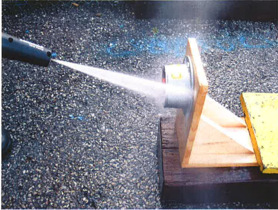
Figure 3A : Pressure-washer resistance test set-up
