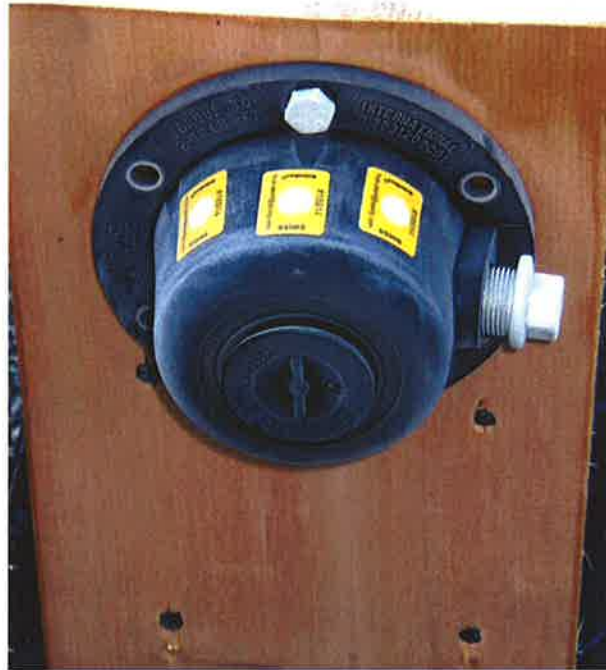
Figure 17A : Plastic hub cap with labels – Cold temperature, before pressure spraying
