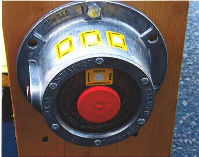
Figure 19A : Aluminum hub cap with labels – Cold temperature, after pressure spraying
