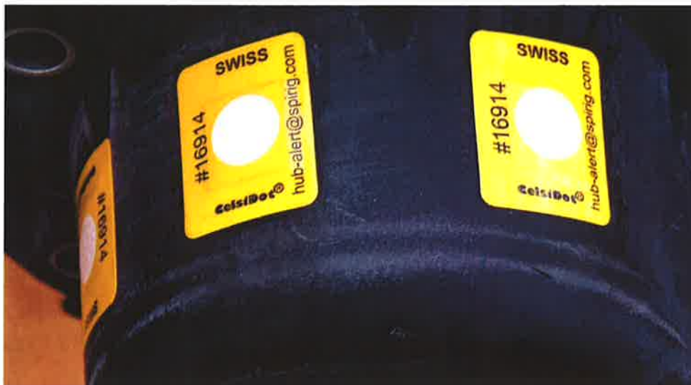
Figure 8A : Plastic hub cap with labels – Ambient temperature, after pressure spraying
