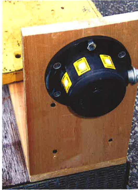
Figure 5A : Plastic hub cap with labels – Ambient temperature, before pressure spraying
